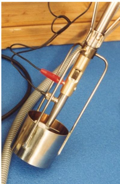
The flow-log type PV is used to measure the speed of the flow in a bore hole.
