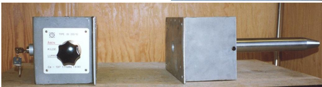
Example of a density probe. The density of the materials between the 2 boxes is measured with a great accuracy. NUCLETRONICS also has equipment for measure the density of brake pads and also weight on conveyer belt is available. The weight on conveyer belt is interestingly for materials with low weight i.e. isolating materials as LECA.
